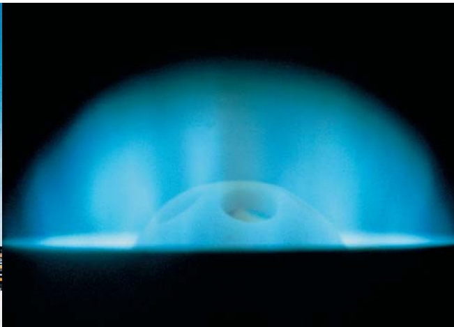
Complete combustion of \text{Cl}_2 and \text{H}_2 in an HCl synthesis burner to produce HCl
