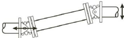
Hinged and slotted FLUROFLEX® bellows allow axial movement of the bellow in addition to angular movement.
